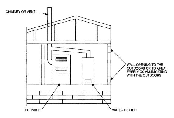
For SI: 1 square inch = 645.16 mm<sup>2</sup>, 1 British thermal unit per hour = 0.2931 W. NOTE: Each opening shall have a free area of not less than 1 square inch per 4,000 Btu/h of the total input rating of all appliances in the enclosure.
