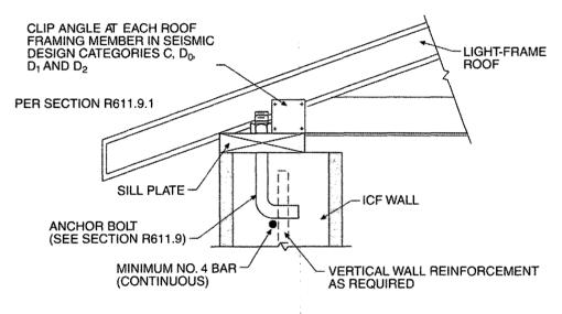
NOTE: Section cut through flat wall or vertical core of a waffle- or screen-grid wall.
