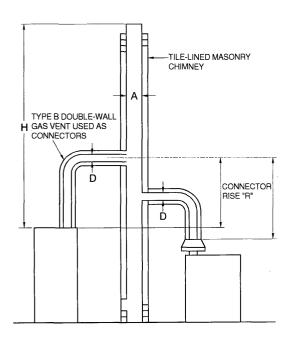
Table G2428.3(3) is used when sizing Type B double-wall vent connectors attached to a tile-lined masonry chimney.
