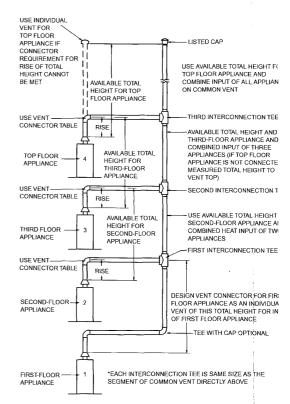
Principles of design of multistory vents using vent connector and common vent design tables (see Sections G2428.3.11 through G2428.3.13).
