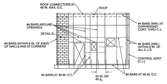
MINIMUM REINFORCEMENT FOR MASONRY WALLS
