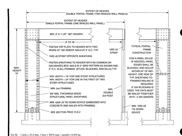
studs. The bearing studs shall also have a tie-down device fastened to the foundation with an uplift capacity of not less than 1000 pounds (4448 N).
