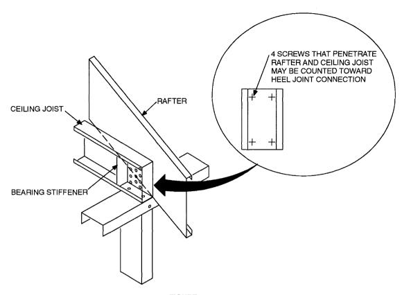
FIGURE R804.3.8 BEARING STIFFENER
