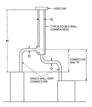
Table G2428.3(2) is used when sizing single-wall vent connectors attached to a Type B double-wall common vent.
