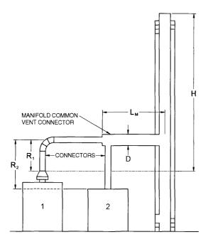
Example: Manifolded Common Vent Connector  $L_{\rm M}$  shall be no greater than 18 times the common vent connector manifold inside diameter; i.e., a 4-inch (102 mm) inside diameter common vent connector manifold shall not exceed 72 inches (1829 mm) in length (see Section G2428.3.4).
