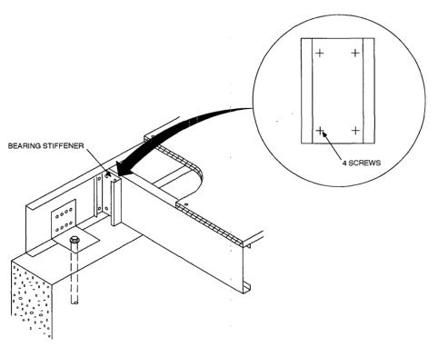
FIGURE R505.3.4 BEARING STIFFENER
