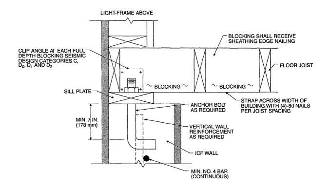
FIGURE R611.8(6) ANCHORAGE REQUIREMENTS FOR TOP BEARING WALLS FOR TOWNHOUSES IN SEISMIC DESIGN CATEGORY C AND ALL BUILDINGS IN SEISMIC DESIGN CATEGORIES  $D_0$ ,  $D_1$ , AND  $D_2$  FOR FLOOR FRAMING PARALLEL TO WALL
