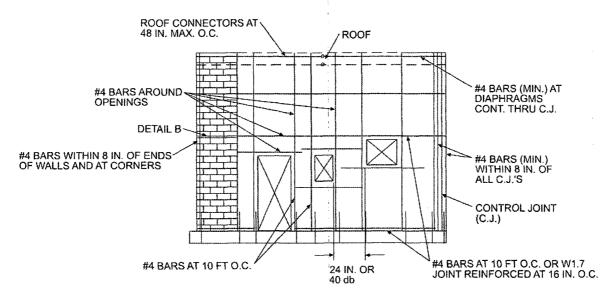
MINIMUM REINFORCEMENT FOR MASONRY WALLS
