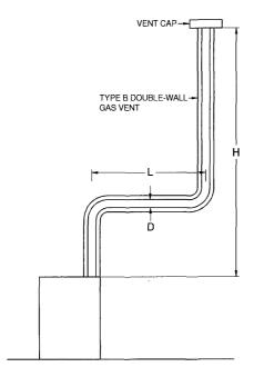
For SI: 1 foot = 304.8 mm, 1 British thermal unit per hour = 0.2931 W. Table G2428.2(1) is used when sizing Type B double-wall gas vent connected directly to the appliance.
