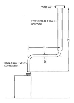
For SI: 1 foot = 304.8 mm, 1 British thermal unit per hour = 0.2931W. Table G2428.2(2) is used when sizing a single-wall metal vent connector attached to a Type B double-wall gas vent.
