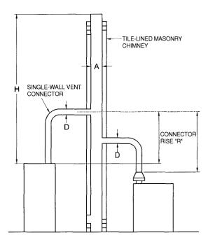
Table G2428.3(4) is used when sizing single-wall metal vent connectors attached to a tile-lined masonry chimney.
