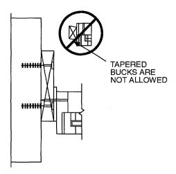
THROUGH THE FRAME ANCHORING METHOD. ANCHORS SHALL BE PROVIDED TO TRANSFER LOAD FROM THE WINDOW OR DOOR FRAME INTO THE ROUGH OPENING SUBSTRATE.
