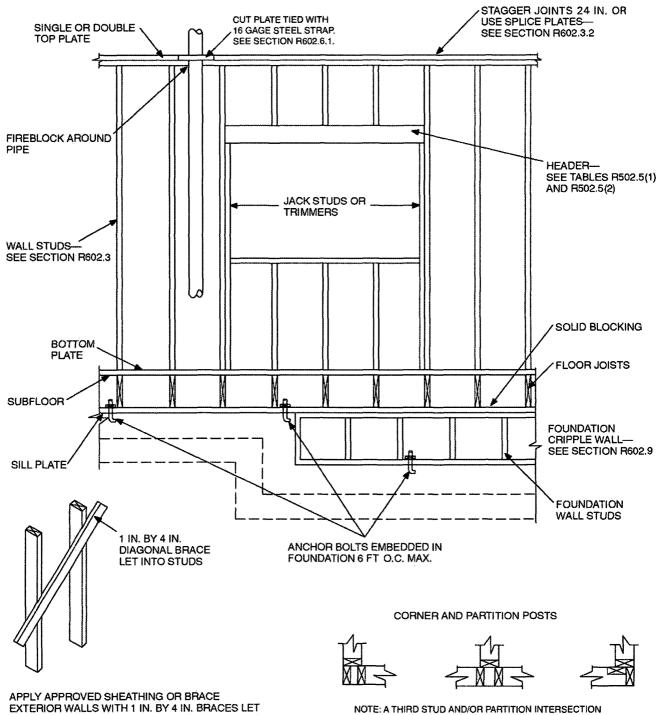
EXTERIOR WALLS WITH 1 IN. BY 4 IN. BRACES LET INTO STUDS AND PLATES AND EXTENDING FROM BOTTOM PLATE TO TOP PLATE, OR OTHER APPROVED METAL STRAP DEVICES INSTALLED IN ACCORDANCE WITH THE MANUFACTURER'S SPECIFICATIONS. SEE SECTION R602.10.
