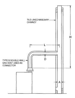
Table 504.2(3) of the *International Fuel Gas Code* is used when sizing a Type B double-wall gas vent connector attached to a tile-lined masonry chimney.
