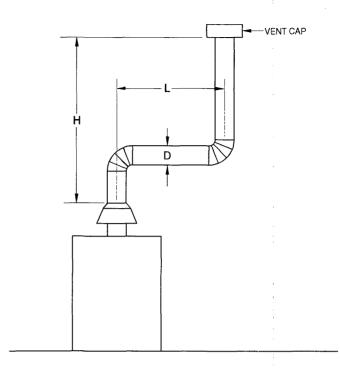
Asbestos cement Type B or single-wall metal vent serving a single draft-hood-equipped appliance [see Table 504.2(5) of the *International Fuel Gas Code*].
