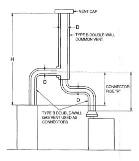
Table G2428.3(1) is used when sizing Type B double-wall vent connectors attached to a Type B double-wall common vent.
