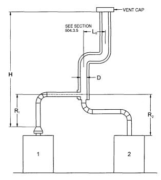
Asbestos cement Type B or single-wall metal pipe vent serving two or more draft-hood-equipped appliances [see Table 504.3(5) of the *International Fuel Gas Code*].
