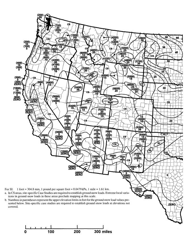
FIGURE R301.2(5) GROUND SNOW LOADS,  $P_g$ , FOR THE UNITED STATES (Ib/ft²)
