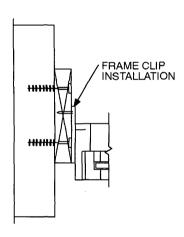
APPLY FRAME CLIP TO WINDOW OR DOOR FRAME IN ACCORDANCE WITH PUBLISHED MANUFACTURER'S RECOMMENDATIONS. ANCHORS SHALL BE PROVIDED TO TRANSFER LOAD FROM THE FRAME CLIP INTO THE ROUGH OPENING SUBSTRATE.
