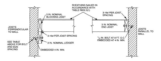
NOTE: Where bolts are located in hollow masonry, the cells in the courses receiving the bolt shall be grouted solid. For SI: 1 inch = 25.4 mm, 1 foot = 304.8 mm, 1 pound per square foot = 0.0479 kPa.
