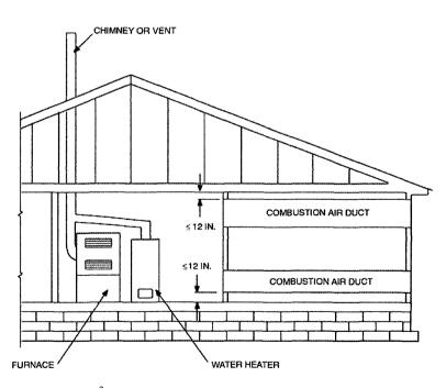
For SI: 1 inch = 25.4 mm, 1 square inch = 645.16 mm<sup>2</sup>, 1 British thermal unit per hour = 0.2931 W. NOTE: Each opening shall have a free area of at least 1 square inch per 2,000 Btu/h of the total input of all appliances in the space.
