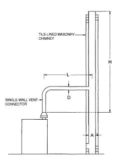
Table 504.2(4) of the *International Fuel Gas Code* is used when sizing a single-wall vent connector attached to a tile-lined masonry chimney.
