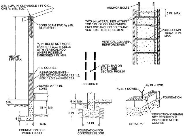
Note: A full bed joint must be provided. All cells containing vertical bars are to be filled to the top of wall and provide inspection opening as shown on detail "A." Horizontal bars are to be laid as shown on detail "B." Lintel bars are to be laid as shown on Section C.
