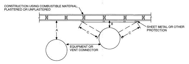
NOTE: "A" equals the required clearance with no protection. "B" equals the reduced clearance permitted in accordance with Table M1306.2. The protection applied to the construction using combustible material shall extend far enough in each direction to make "C" equal to "A."
